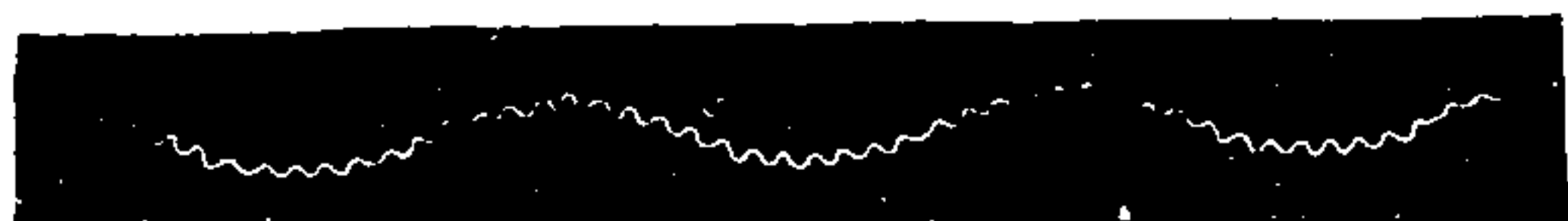
Fig. 53. Vibrations of compound sounds.
