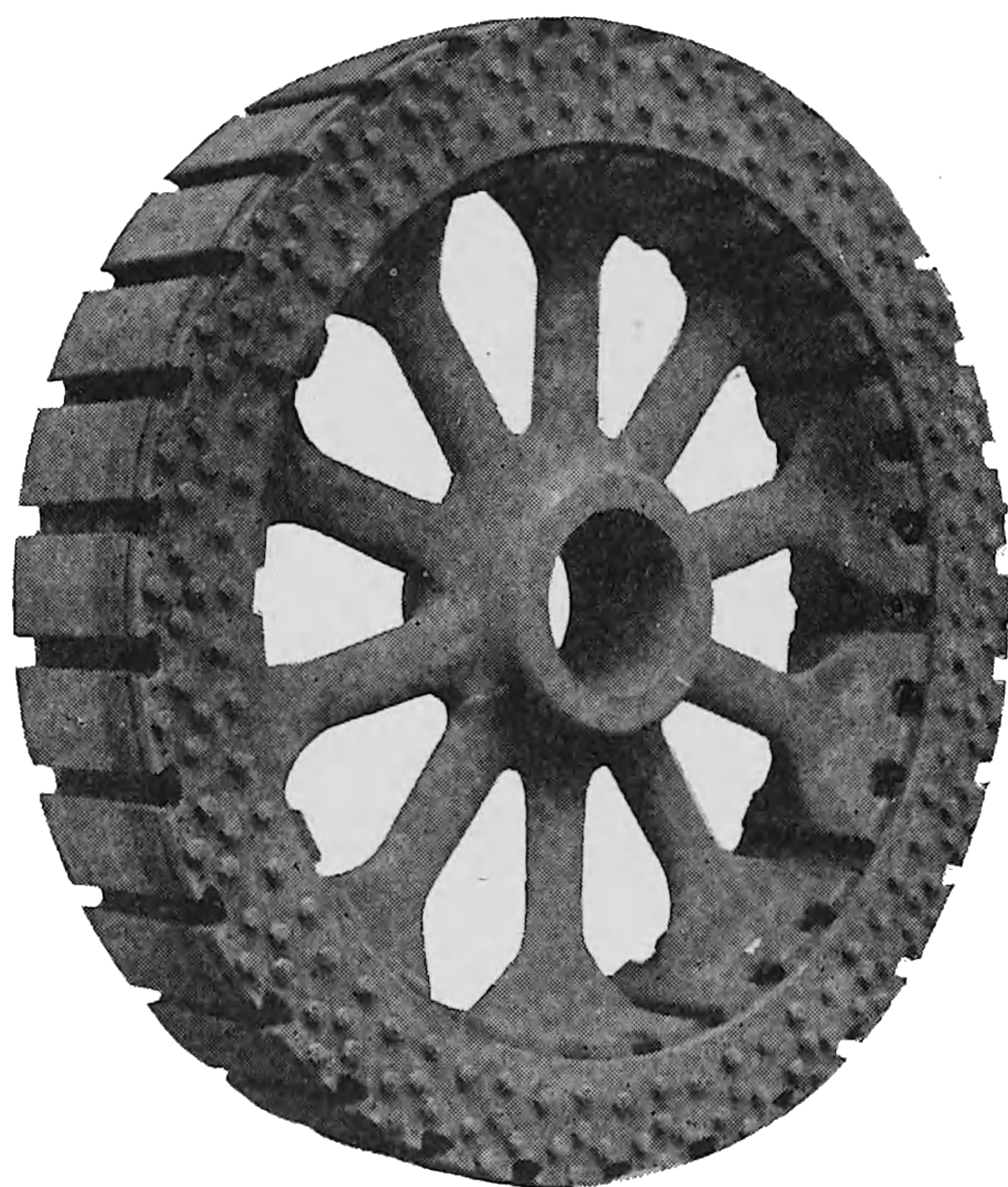
Fig. 166. Westinghouse Rotor Construction Showing Cast Spider, Laminated Rim, and Dovetailed Slots
