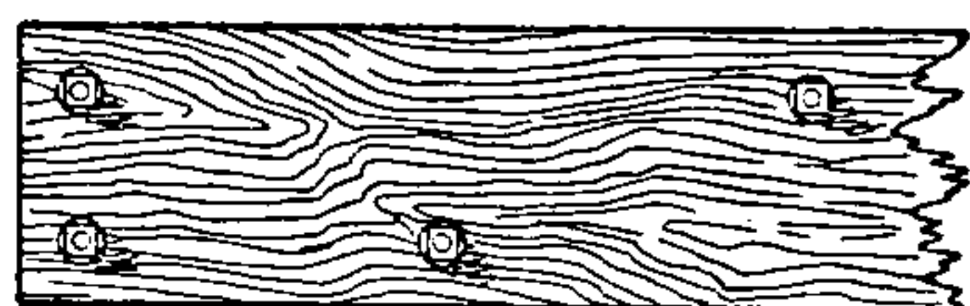
Fig. 227. Construction of Compound Beam
