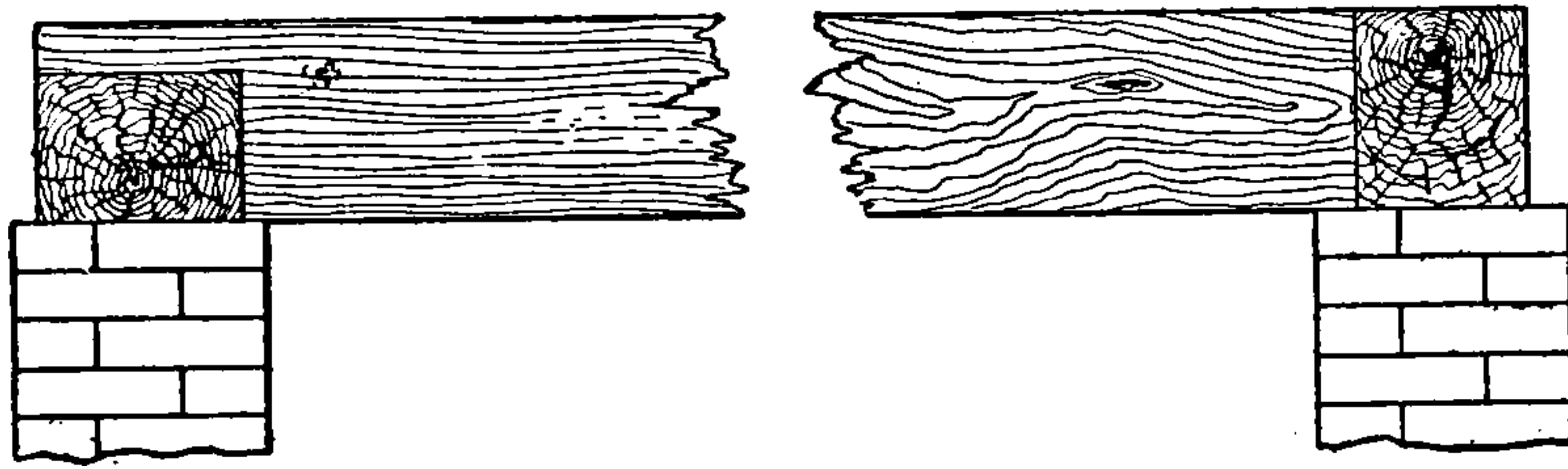
Fig. 150. Superior Floor Joist and Sill Construction
