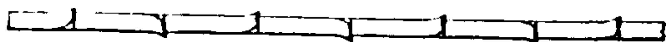
Fig. 20. Blade of Rip Saw Edge-On
