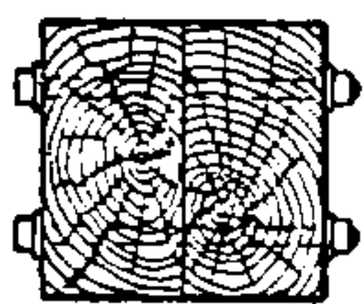
Fig. 227. Construction of Compound Beam
