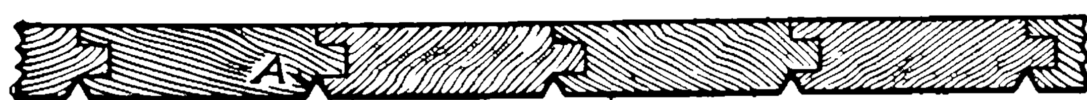
Fig. 357. V-Shaped Sheathing
