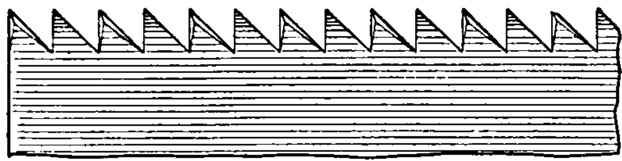
Fig. 24. Slope of Teeth of Back Saw
