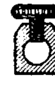
Fig. 23 Circular Shank and Socket
