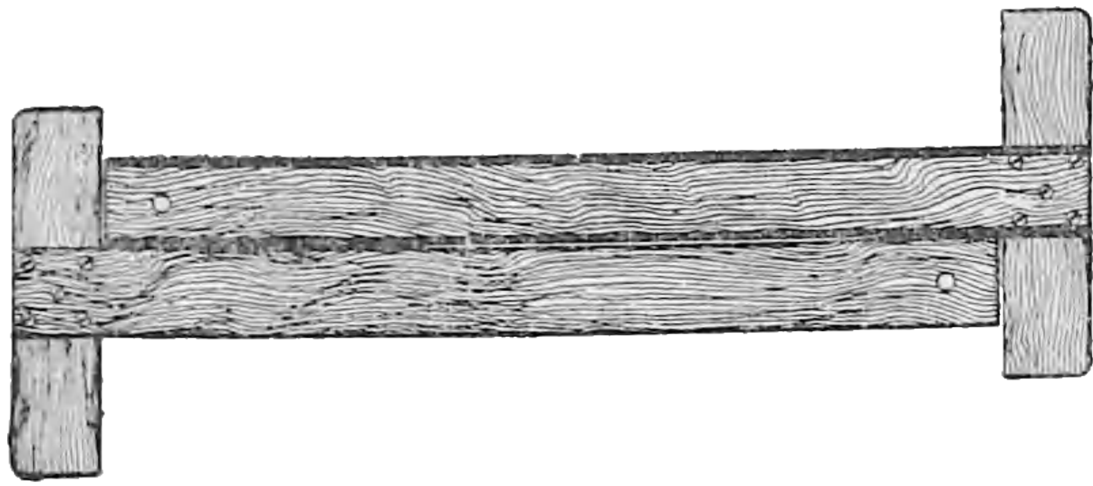
Fig. 8. Testing the Edge of T-Square
