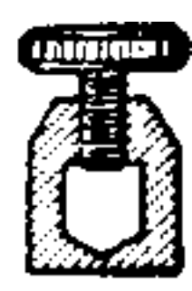
Fig. 22 Pentagonal Shank and Socket
