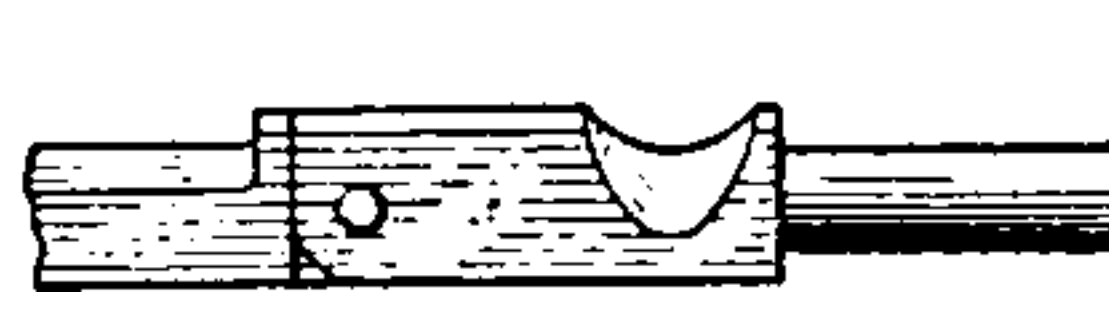
Fig. 23 Circular Shank and Socket
