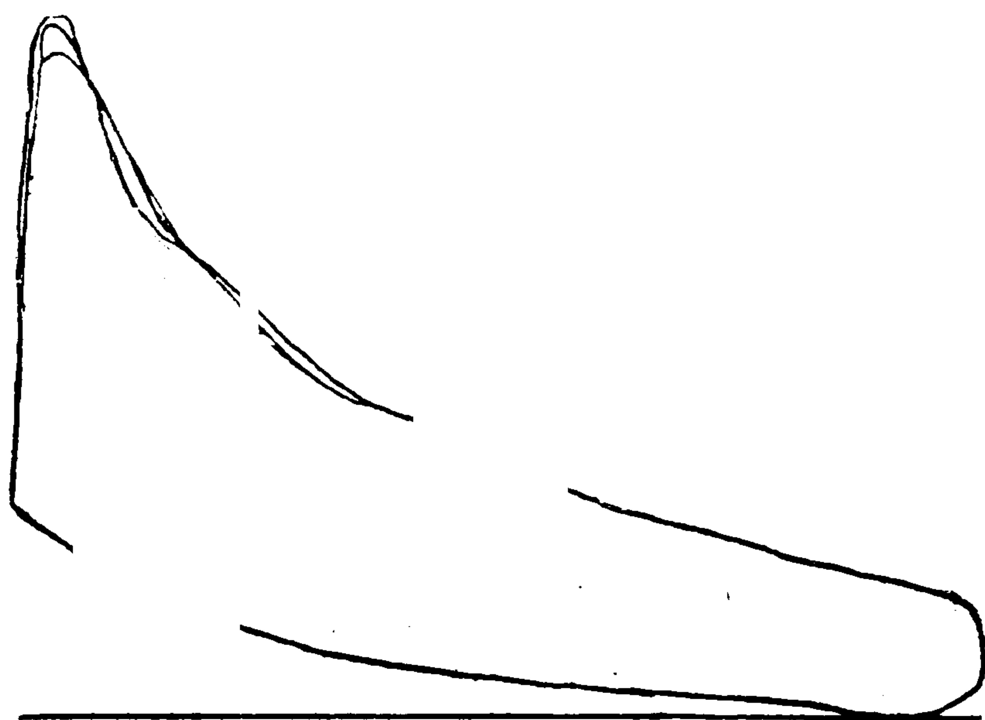
FIG. 11.—TYPICAL COMPRESSION CARD. MEAN PRESSURE, 76 LBS. PER SQUARE INCH.
