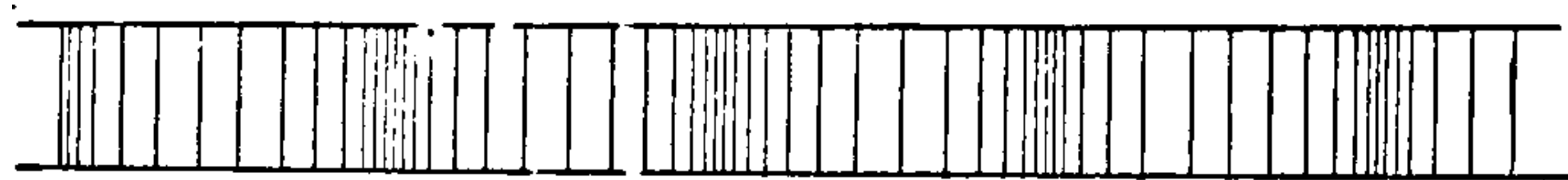
FIG. 143. — Showing the compression and rarefactions in Kundt's tube.
