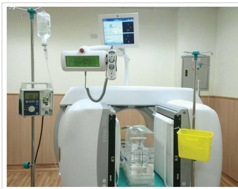
Figure 3. The arrangement of the water phantom between the gamma camera's 2 NaI plates. As previously noted, the container for holding the draining water was kept at the same height as the top of the phantom in order to assure the water balance.
