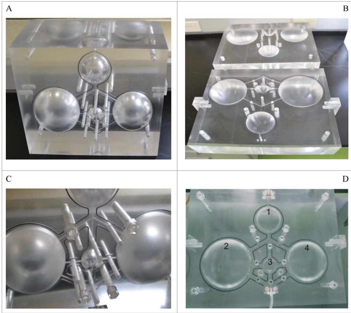
Figure 1. The 2 halves of each acrylic cube: (A) top view of the assembled phantom, (B) split into the completed halves, (C) close-up view of the valve pole in the middle of the ditch between the spherical chambers, and (D) spherical chambers labeled as regions of interest (ROI) (1)–(4).
